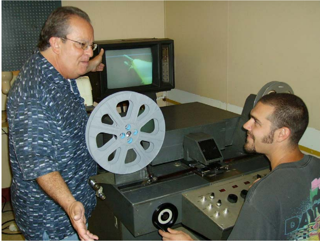
Cinefilm Lab Manager Tony Bifano discusses density settings with color timer Jason Apple. Critical adjustments on the classic Hazeltine color timing system were required to study the detail of debris created by the Shuttle launch.
