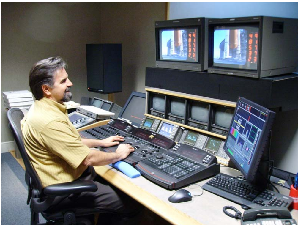
Senior Colorist Ron Anderson makes adjustments to Shuttle launch footage on the Spirit 2K Telecine at Cinefilm in Atlanta. HD transfers were input to the QuVis data system at 1080p.
